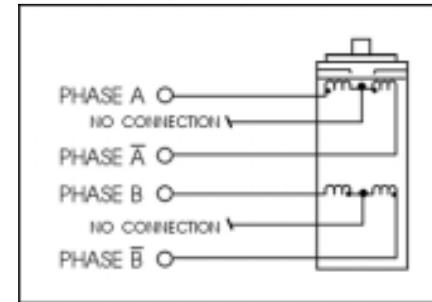
Figure 7: 6 Lead Full Coil (Higher Torque) Motor
