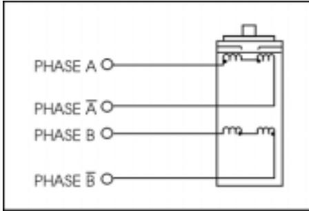
Figure 8: 4 Lead Motor Connections
