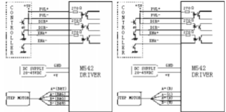
Figure 9: Driver connection in a stepping system
