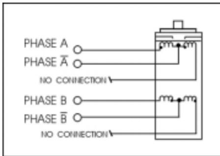
Figure 6: 6 Lead Half Coil (Higher Speed) Motor Connections
