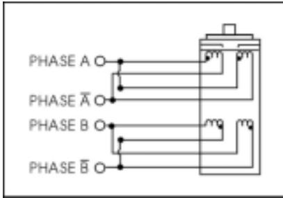
one half of the motor's inductor windings. The higher torque configuration, or full coil, use the full windings of the phases.
